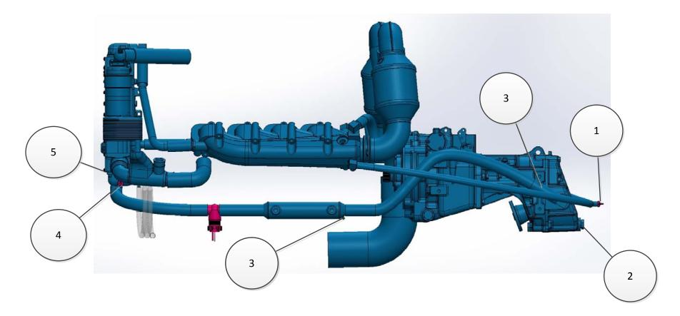
The raw water side of the cooling system is protected from freezing by draining the raw water from the system. The drain points are indicated on the winterization points drawings for Premium and Standard engines.
